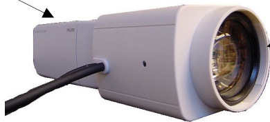
Camera with assembled motorized zoomlens
